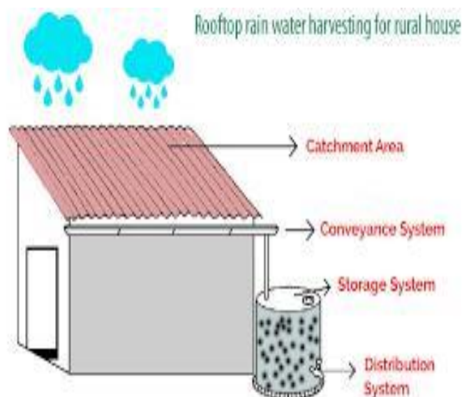
Figure 1. Rainwater harvesting system for house (Ltd., n.d.)
