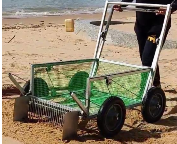
Figure 12. Completed Beach Cleaning Machine
