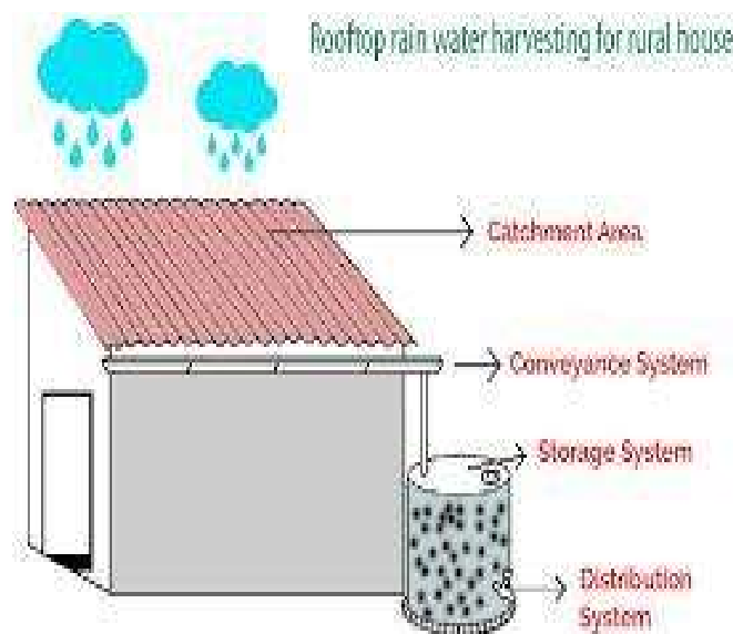
Figure 1. Rainwater harvesting system for house (Ltd., n.d.)
