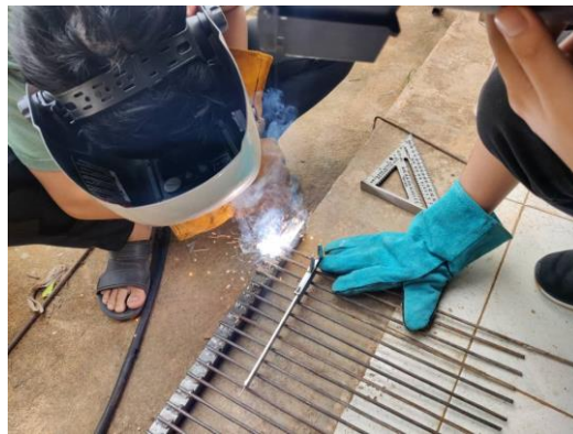
Figure 9. Weldment Process of Rake
